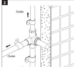
Install the valve with proper fitting or use mounting holes on valve. Support as noted in image. Turn on water supply and inspect for leaks.
