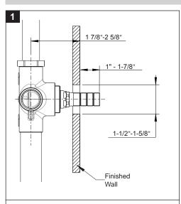
Position valve according to measurements noted in
