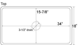
Dimensions of fixture are nominal and may vary within the range of tolerances established by ANSI Standard A112.19.22.2013 Dimensions and specifications subject to change without notice.
